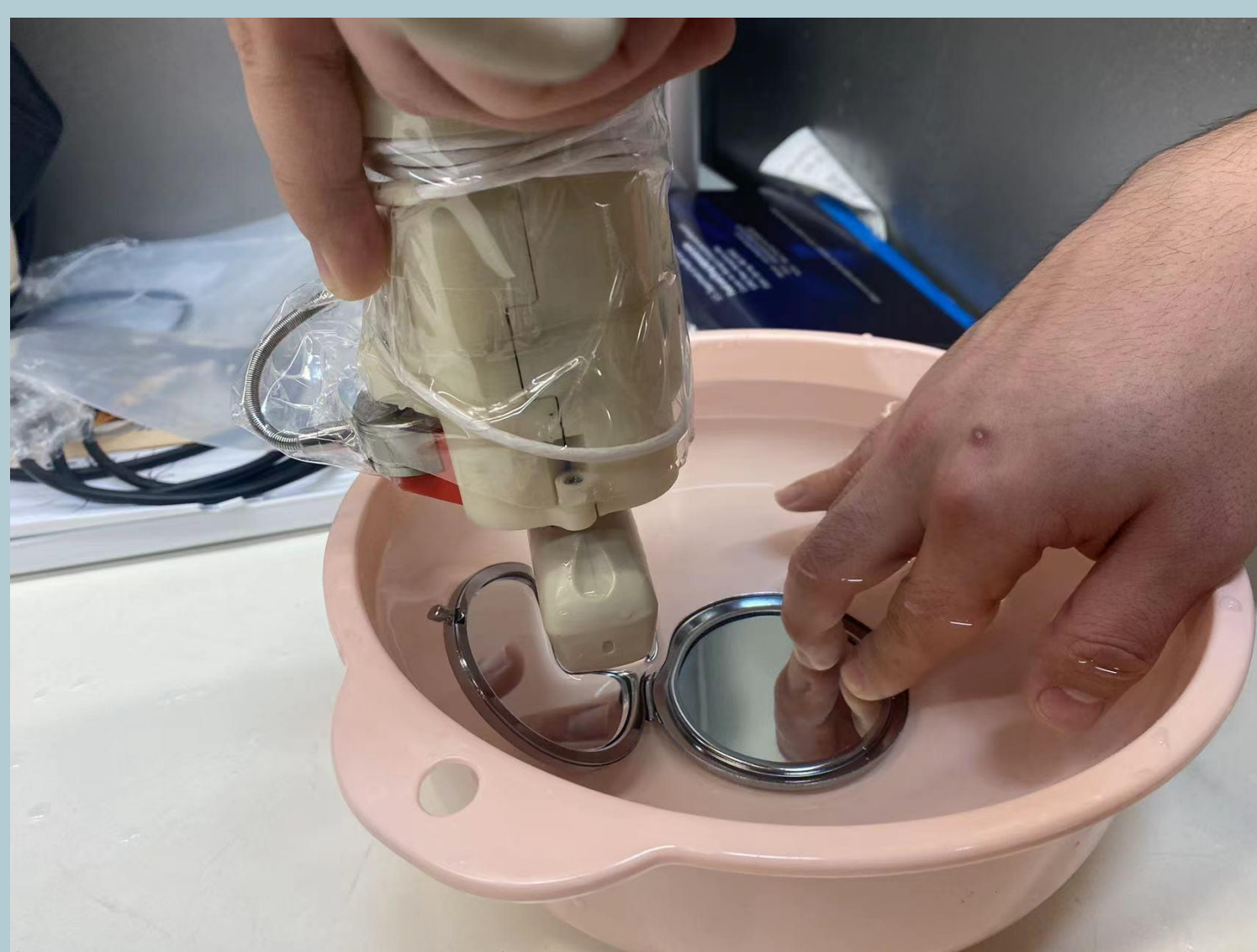
Figure 1 (a): We placed a mirror in the water to test if the ultrasound image could be captured after the ultrasound waves were reflected.
