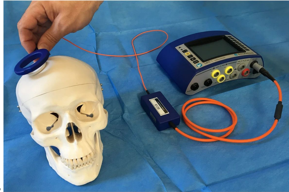
Illustrating the NEUROVENT® ICP-Monitoring System and its approximate relation to the skull during ICP monitoring [1]
