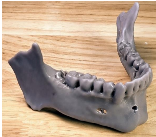
Figure 4. 3D Printed Mandible Phantom.
