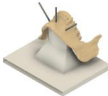
Figure 3. Mandible oriented onto mounting setup.
