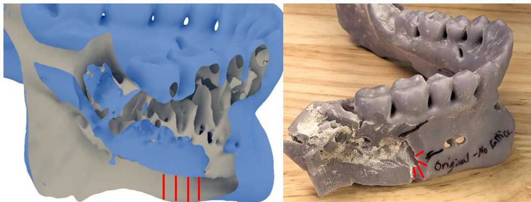
Figure 5. Thick cortical bone in original segmentations.
