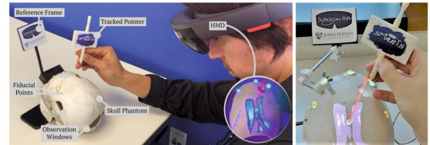
Fig. 1. Left: User wearing HMD and holding tracked pointer to perform registration. Right: Updated skull phantom (new fiducials, reference frame attachment and borescope cameras for measurement).
