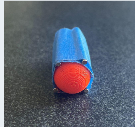
Figure 9: Magnets Around PillCam
