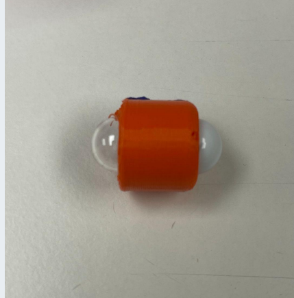
Figure 8: Magnet Housing with PillCam
