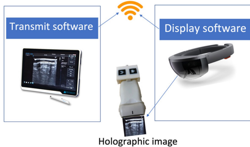
Fig. 1 Two main software modules of the HoloUS app: the transmit and display modules. The ultrasound image is displayed virtually inside the HoloLens
