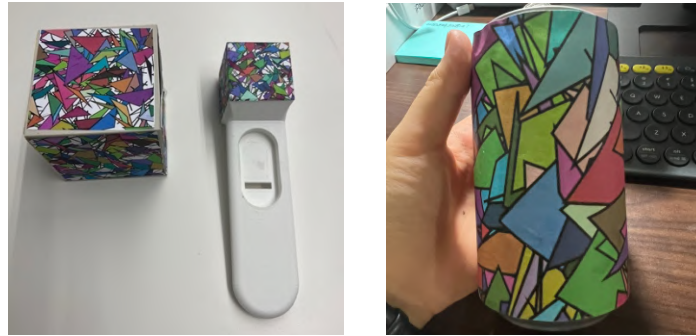
Figure 5. 3D markers for tracking. (Left) Cube marker. (Right) Cylinder marker
