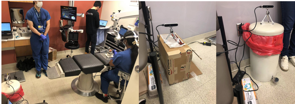
Figure 10. Eggshell Drilling Experiment Setup Figure 11. RGBD depth camera (in two positions)
