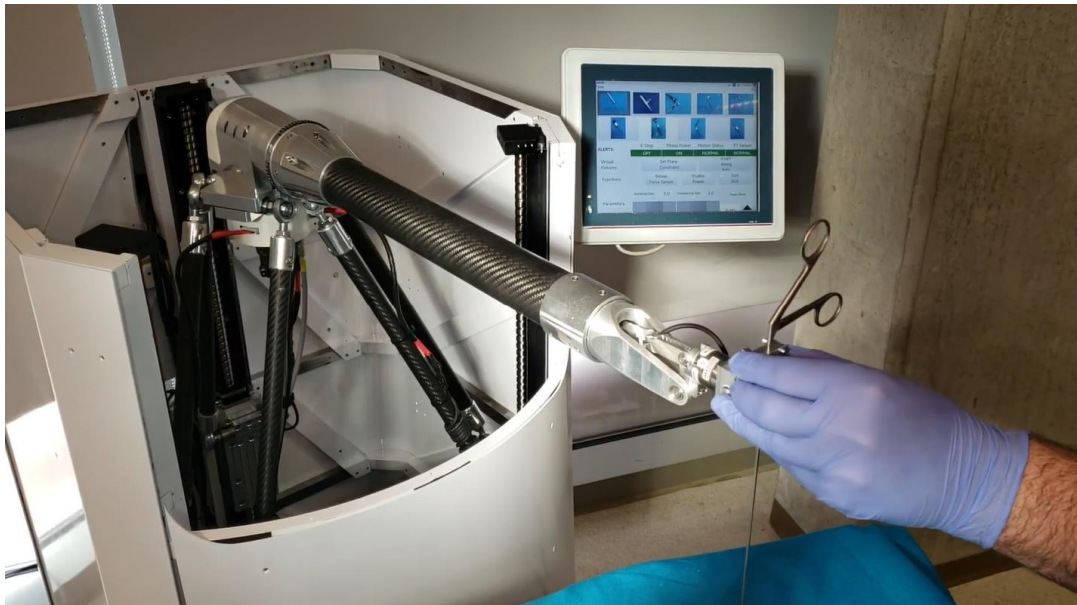
Figure 1 The Galen Robotic System with a tool attached to the End Effector and an operator manipulating the system [2]
