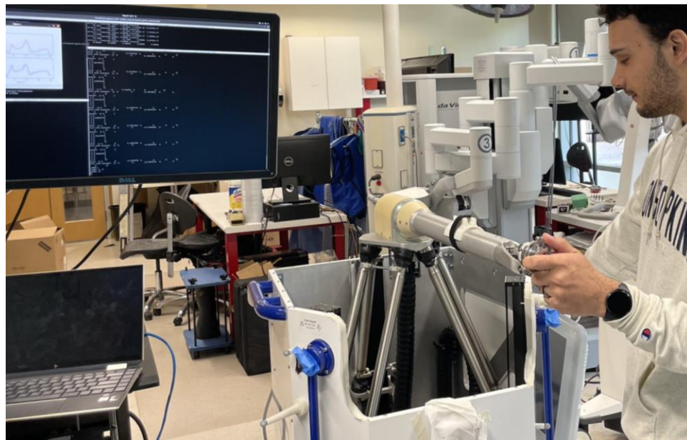
Figure 14 User interacting with the Galen robot end effector to apply a wrench
