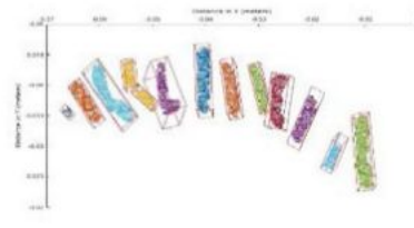
(c) 3D point cloud associated with each stitch. Distances between stitches can be measured by the centroids of adjacent boxes.
