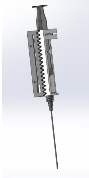
Figure 5: Details of the needle insertion actuator
