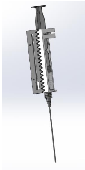
Figure 6: Details of the needle insertion actuator
