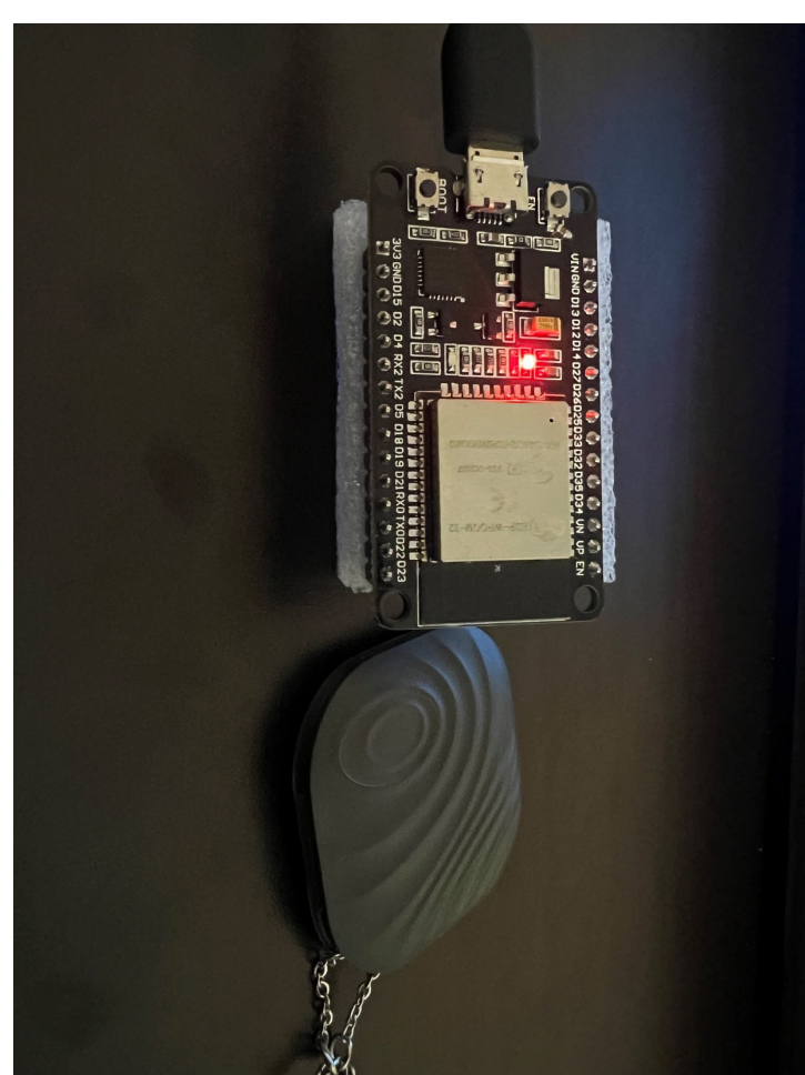
ESP32 Microprocessor (Top) and Nutale BLE Tag (Bottom) Used for Bluetooth Proximity Sensing
