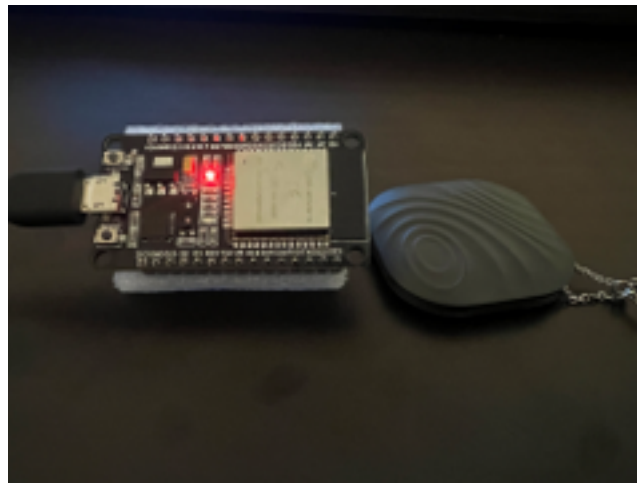
Figure 4: ESP32 Microprocessor (Left) and Nutale BLE Tag (right) Used for Bluetooth Proximity Sensing
