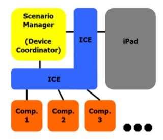
Figure 2: The schematics of our application. The iPad is connected through ICE to the Scenerio Manager, which is then connected through ICE to the various components that we wish to control.
