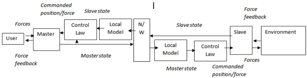
Fig. 6: Block Diagram of Teleoperation Architecture.
