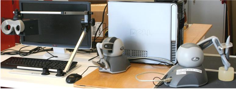
(a) The Sensable Omni Master/Slave Setup with a Stereo Viewer
