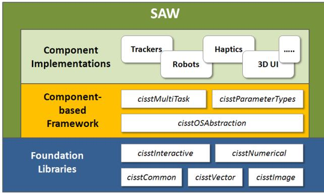
Fig. 1: SAW Components
