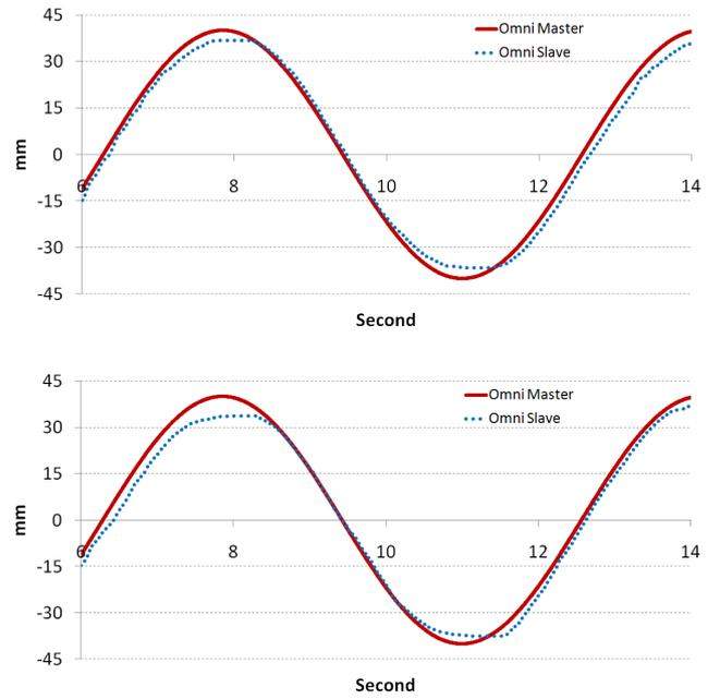
Fig. 7: Position tracking for Omni master and slave manipulators for line movement (left) and sinusoidal input (right).
