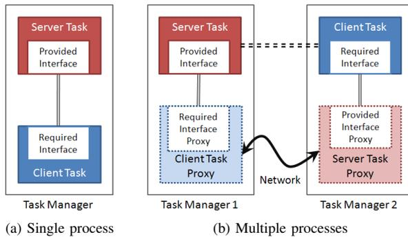
Fig. 3: The Proxy Pattern in the *cisstMultiTask* library
