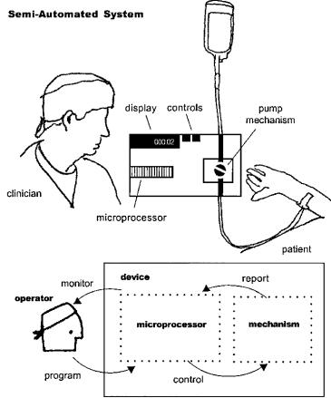
Fig. 1. Infusion device as a manual and semiautomatic system.
