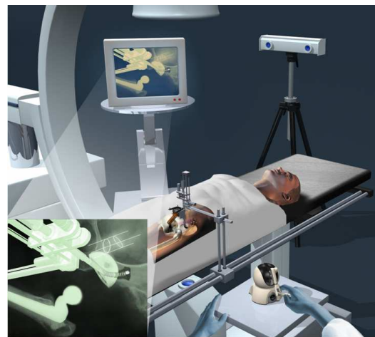
Fig. 1. Conceptual depiction of revision surgery highlighting the acetabular shell with removed polyethylene liner, and the dexterous manipulator accessing an osteolytic lesion through a screw hole.
