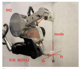
Figure 2 - RND robot showing ideal rotation axes and needle path
