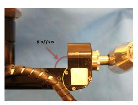
Figure 7 - Adjusting  $\beta$  will help the needle path intersect Rz.
