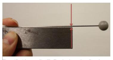
Figure 12 - A bent needle will affect the observed needle path.
