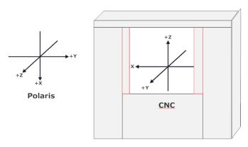
Figure 3 - Coordinate system definitions for Polaris observed and CNC reference coordinates
