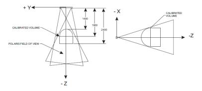
Figure 5 - Tracker geometry as stated in NDI Manual, units in mm.
