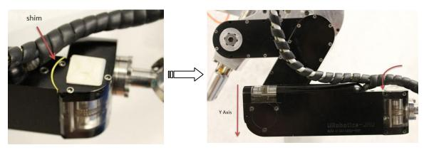
Figure 8 - The shim pushes Rx down to meet Rz.
