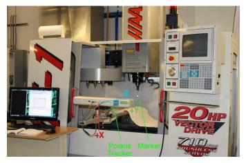
Figure 4 - Polaris 3D test setup
