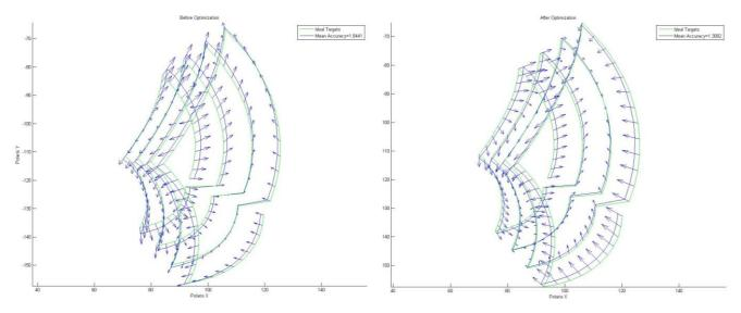
Figure 13 - Visualization of targeting errors before and after parameter optimization
