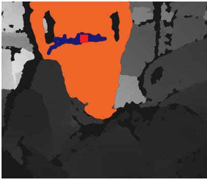
Fig. 6. Example image and temporal segmentation from the second dataset. The orange part represents the image segmentation at this frame, the red square is the current center of mass, and the blue line is the center of mass at each time step in the sequence.
