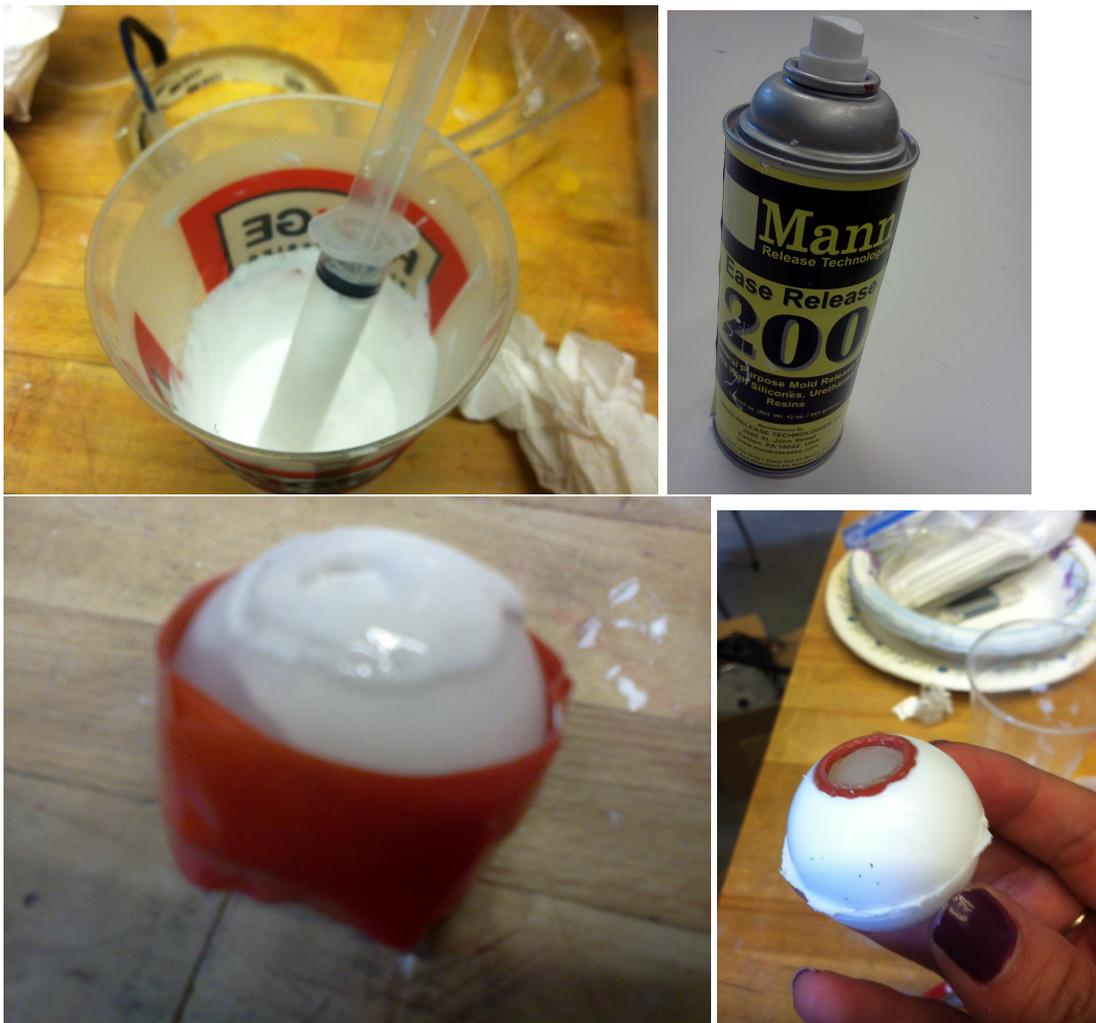
The outer casing is removed and the O-ring carefully removed. The phantom is stretched to removed the inner plastic ball, and finally the O-ring is glued
