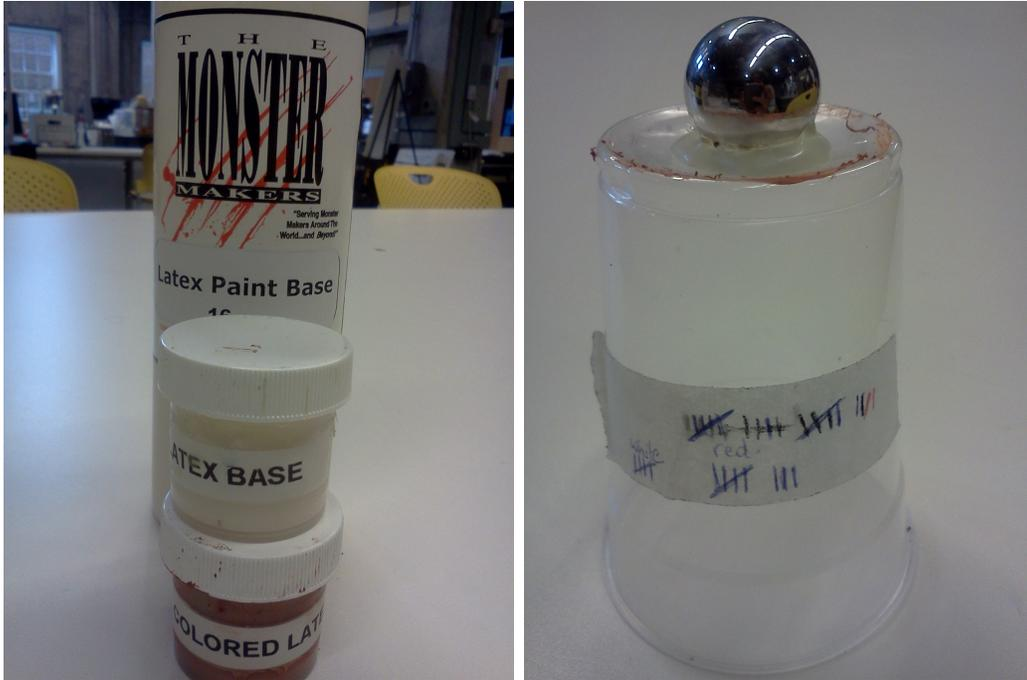
First the ball is dipped into the latex paint base and then allowed to dry over 10 to 15 minutes. Two such layers are done before drawing on the vessels using a fine tipped pen. The drawn on vessels were allowed to dry for 24 hours, then dabbed with tissue paper to avoid ink bleeding in subsequent dippings.
