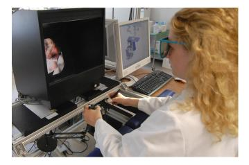
Fig. 2. Master console with Phantom<sup>TM</sup> devices and 3D screen
