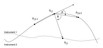
Fig. 4. Directional change of one instrument ( $\rho$ ) and directional change of one instrument w.r.t to a second instrument ( $\theta$ ).
