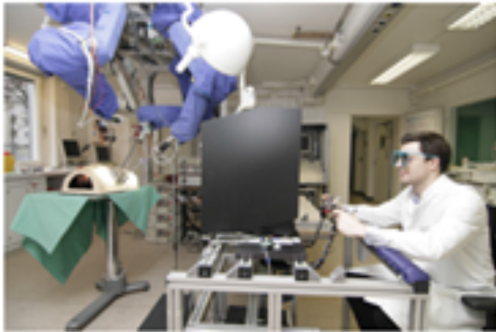
Fig. 1. Hardware setup: Ceiling mounted robots with surgical instruments
