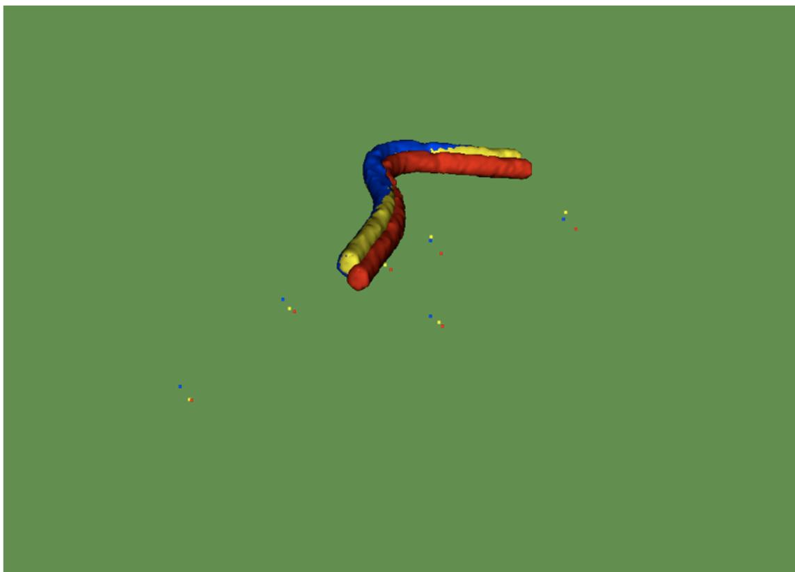
Figure 15: Example of an error reduction from 5.37103 mm to 0.674765 mm with 40 points collected with the 'laser' over the entire surface of the artery. Blue corresponds to ground truth, red corresponds to error, and yellow corresponds to the result following correction.
