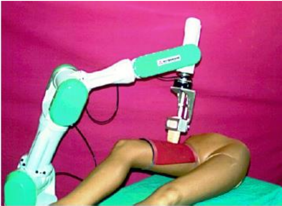
Figure 4. Testbed for force control.
