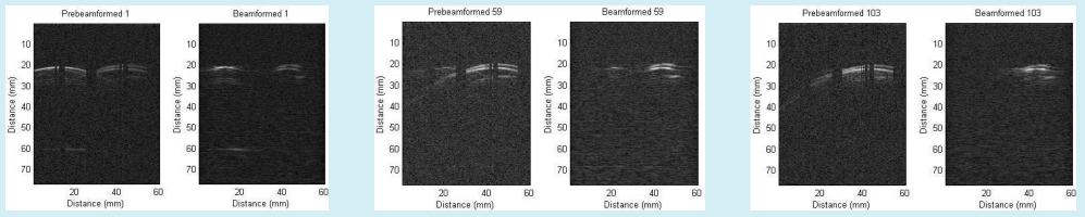
PA image of occlusion and fiber end point with a distance of 20mm (Left), 12mm(Middle), 5mm(Right)
