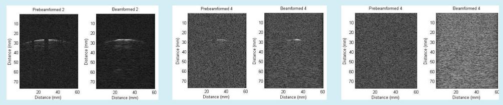
PA image of 4mm thickness occlusion with 2mm pig (Left), 1.5mm thickness (Middle), and no occlusion (Right).
