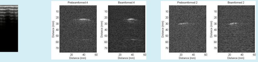
B-mode ultrasound image with 2mm pig bone (Left). PA image with 2mm (Middle) and 4mm (Right) pig bone.
