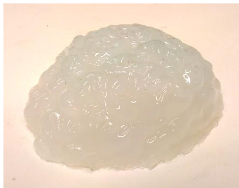
Figure 5: Brain shaped PVA-C phantom
