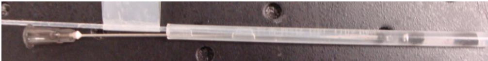
Figure 11: Fiber tied up together with needle and a piece of occlusion material
