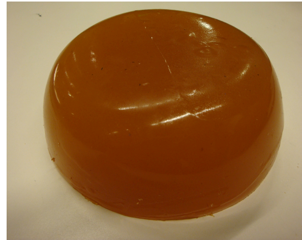
Gelatin and Fiber phantom (Relatively soft, Tissue-like)
