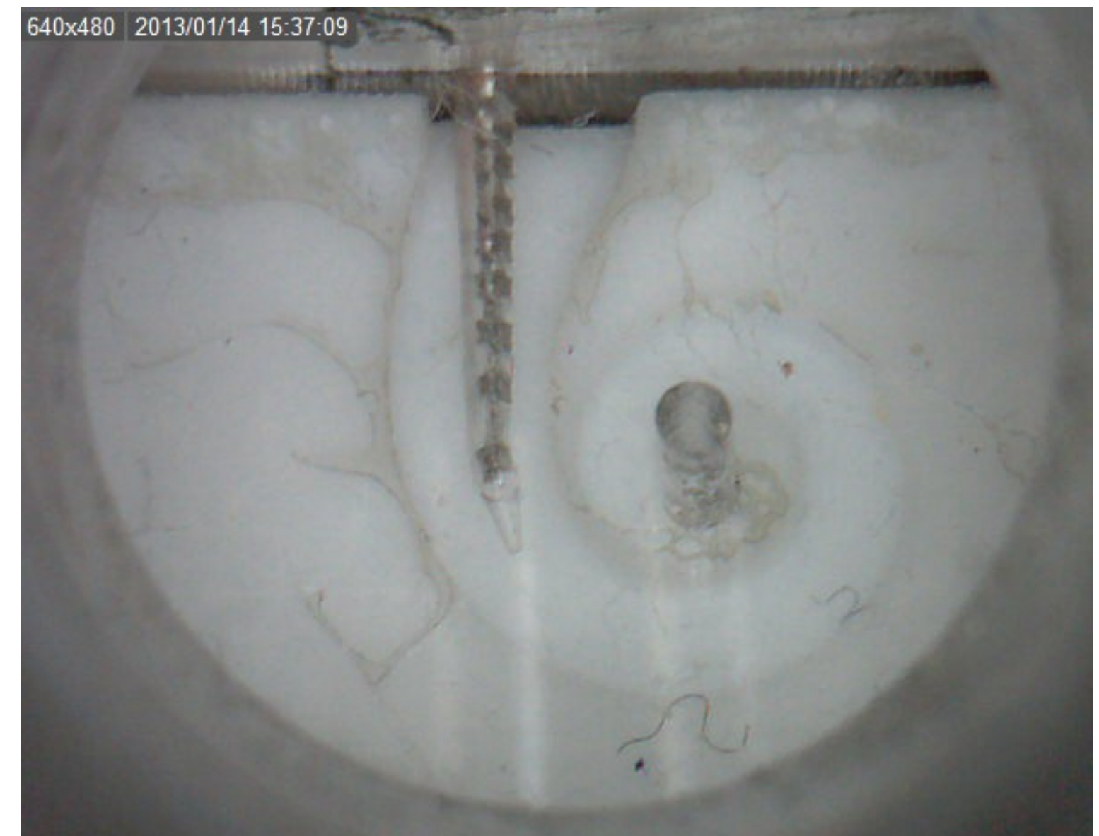
Cochlear Implant in Phantom Cochlea Positioned at Optimal Depth of Insertion
