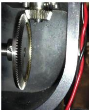
work properly. The adjoining figure shows the same. This causes the encoder reading to overshoot and hence doesn't stop the motor. The Motor E also has similar problem, but the gears haven't slipped yet.
