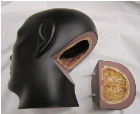
'scarecrow' brain phantom Image provided by the I-star lab
