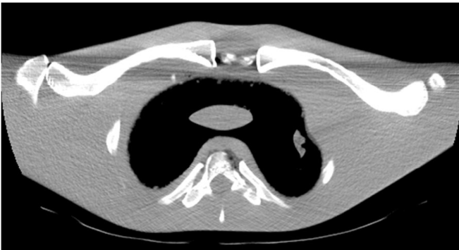
CT image of a shoulder phantom shows streaking artifacts caused by photon starvation. Image provided by Barrett and Keat, Artifacts in CT: Recognition and Avoidance
