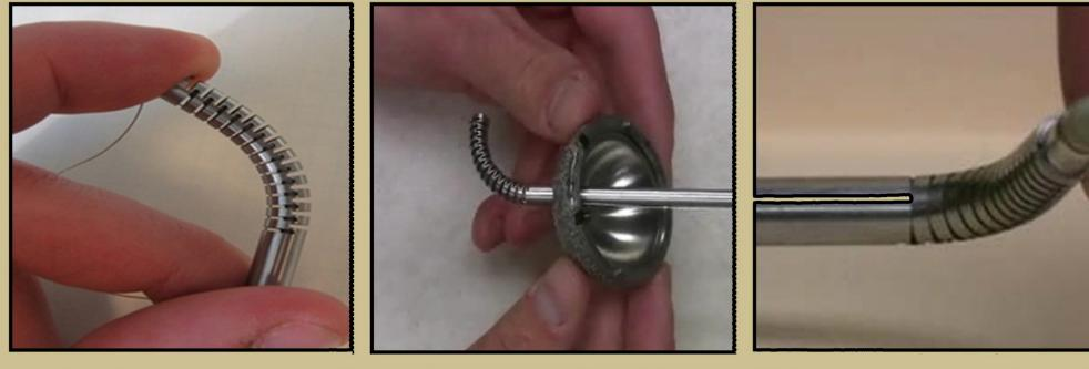
• In the envisioned application, the SDM will be positioned in the workspace by a robotic arm and uses screw holes in the acetabular implant as its entry to the patient's body
