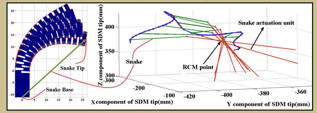
We considered a 3D path for the snake that is a specific boundary of a simulated lesion and is inside a confined cubic space with sides of 7 cm. Optimization result for configuration (Left) and orientation of the snake and actuation unit (Right) in some points of the desired path have been shown. The result shown here means that the robot changes its configuration such that with minimum joint movements the desired goal could be achieved while RCM constraint has been satisfied.
