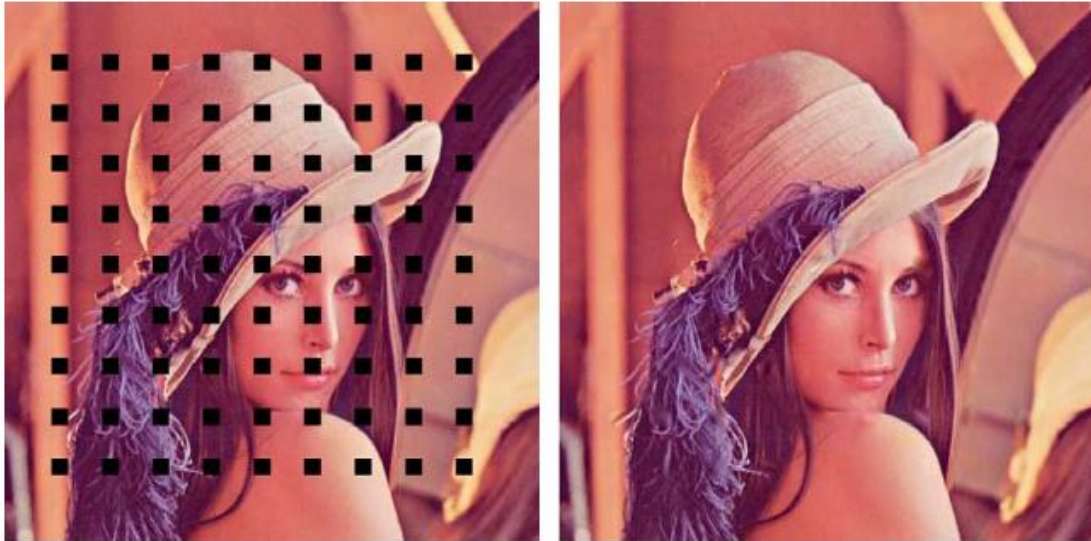
Figure 6 Concealment of block losses using the frequency selective extrapolation technique. Left: Isolated 16 \times 16 block losses. Right: Concealed image; Adapted from Figure 5 of Kaup et al. (2005)
