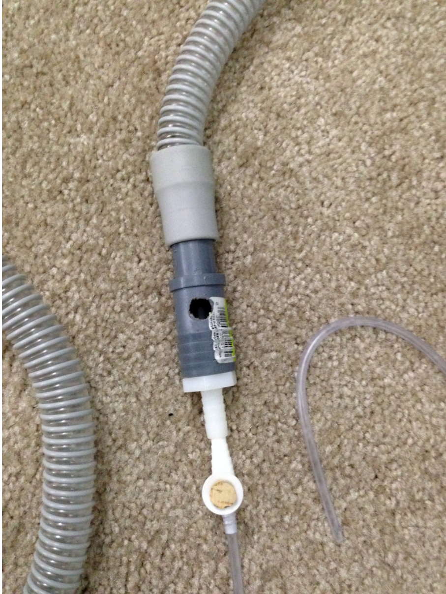
Figure 7: Opening for finger-valve placement
