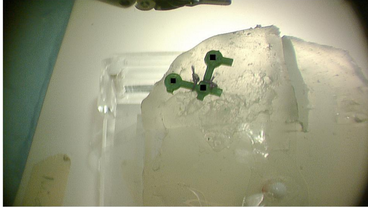
Figure 6 Fiducial detection. The center of each square is the detected fiducial center, and the half length of the square is the detected fiducial radius
