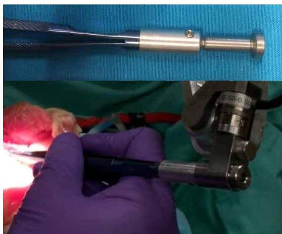
Figure 5: Adapter for needle drivers. Shown both apart and attached to the REMS.
