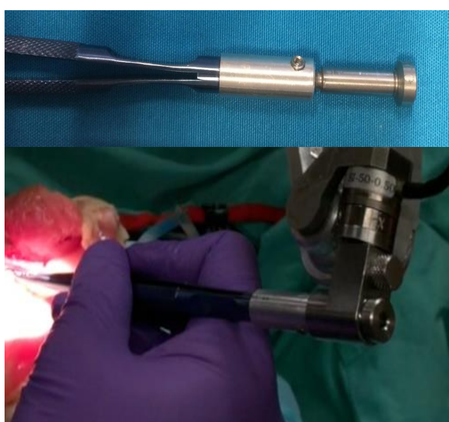
Figure 4: Adapter for needle drivers, apart and attached to the REMS.
