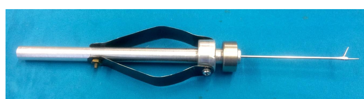
Figure 8: Operational prototype based on design shown in Figure 7. Simplified after difficulty constructing original design, shown in Figure 6.
