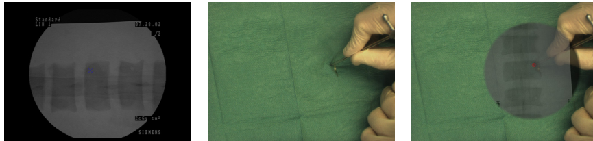
Fig. 1. The CamC system merges the the X-ray image (left) onto the video image (middle), creating an augmented view (right) which provides an intuitive interface for skin incision and instrument positioning.
