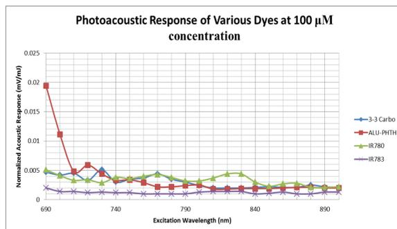
Photoacoustic response spectrums of dyes with absorbance peaks in the near infrared region. For each sample, the output of the hydrophone was divided by the laser's energy at that wavelength to give the normalized response
