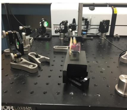
(Left: Full system in use with skull sample) An OPO laser is aimed directly at the well using mirrors. The hydrophone is aimed at the well, at a 90 degree angle to the excitation laser path. The photoacoustic signal is picked up by the hydrophone as the dyes are bombarded by light energy. The hydrophone response is monitored via an oscilloscope (not pictured).
