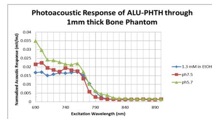
The introduction of a piece of bone between the hydrophone and the phantom seemed to "smooth" the response. The potentially useful local max/min trend at 770 nm disappeared when the bone was introduced
