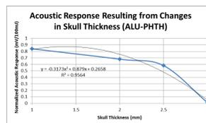
Increasing thicknesses of bone between the hydrophone and gel decreased signal magnitude
