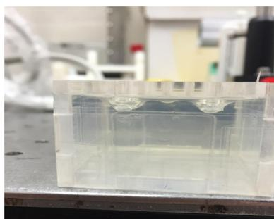
(Left) We designed and iteratively improved a phantom mold, to be cast with porcine gelatin. The phantom contains four separate wells to hold different candidate dyes. The use of cast wells in the aqueous gel creates a nearly homogeneous path for light and acoustic signal transmission, avoiding material transitions common in other phantoms.
