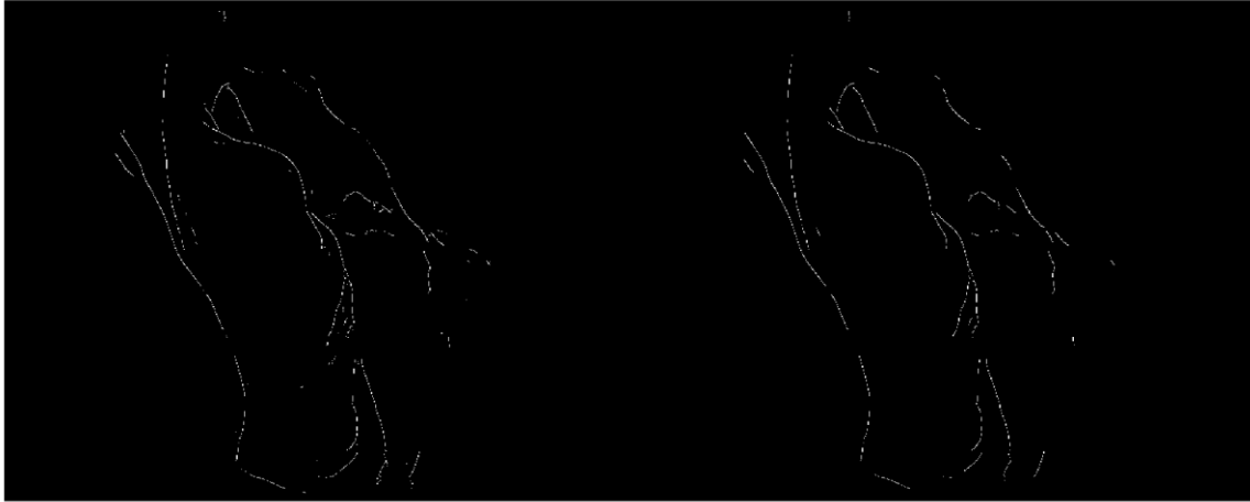
FIGURE 9. LEFT: EDGE DETECTION AFTER USING CANNY FOR PREDICTION. RIGHT: EDGE DETECTION IMAGE AFTER APPLYING CLOSING AND OPENING TO THE LEFT IMAGE.
