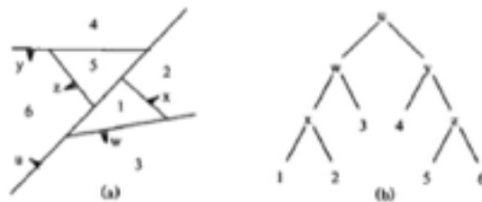
Figure BSPT. Geometry of a 2D partitioning (a) and its BSP tree (b).
