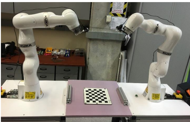
Figure 1: CAMP lab's dual robotic platform with two KUKA iiwa robotic manipulators.
