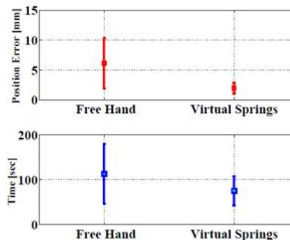
The virtual spring control shows an improvement in both time and accuracy when compared to free hand control
