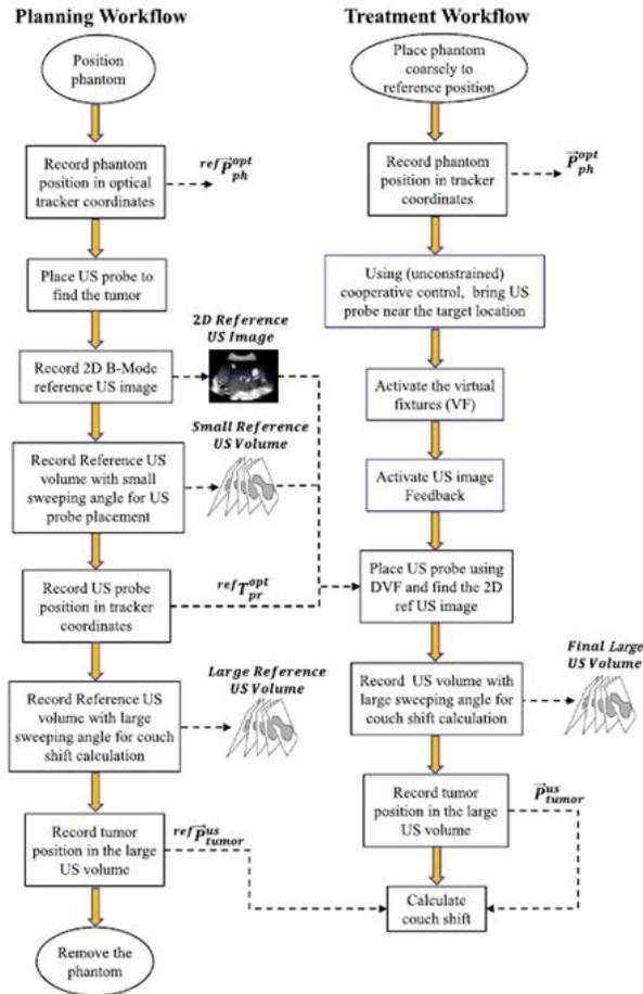
FIGURE 7 | Experiment workflow for testing US image-based patient setup.
