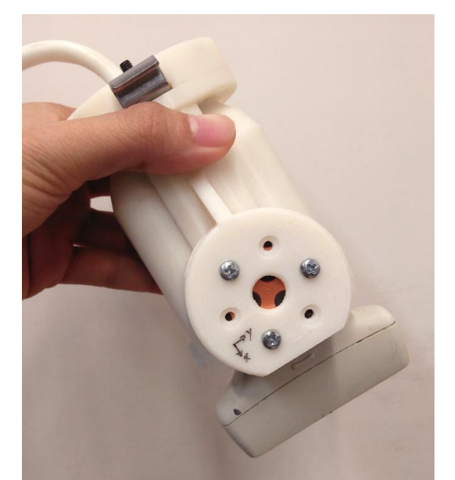
Figure 9. US attachment with 3-axis load cell
