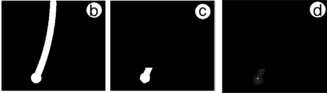
Fig.6 From binary mask to cropped region of interest to prior estimation of tip point
