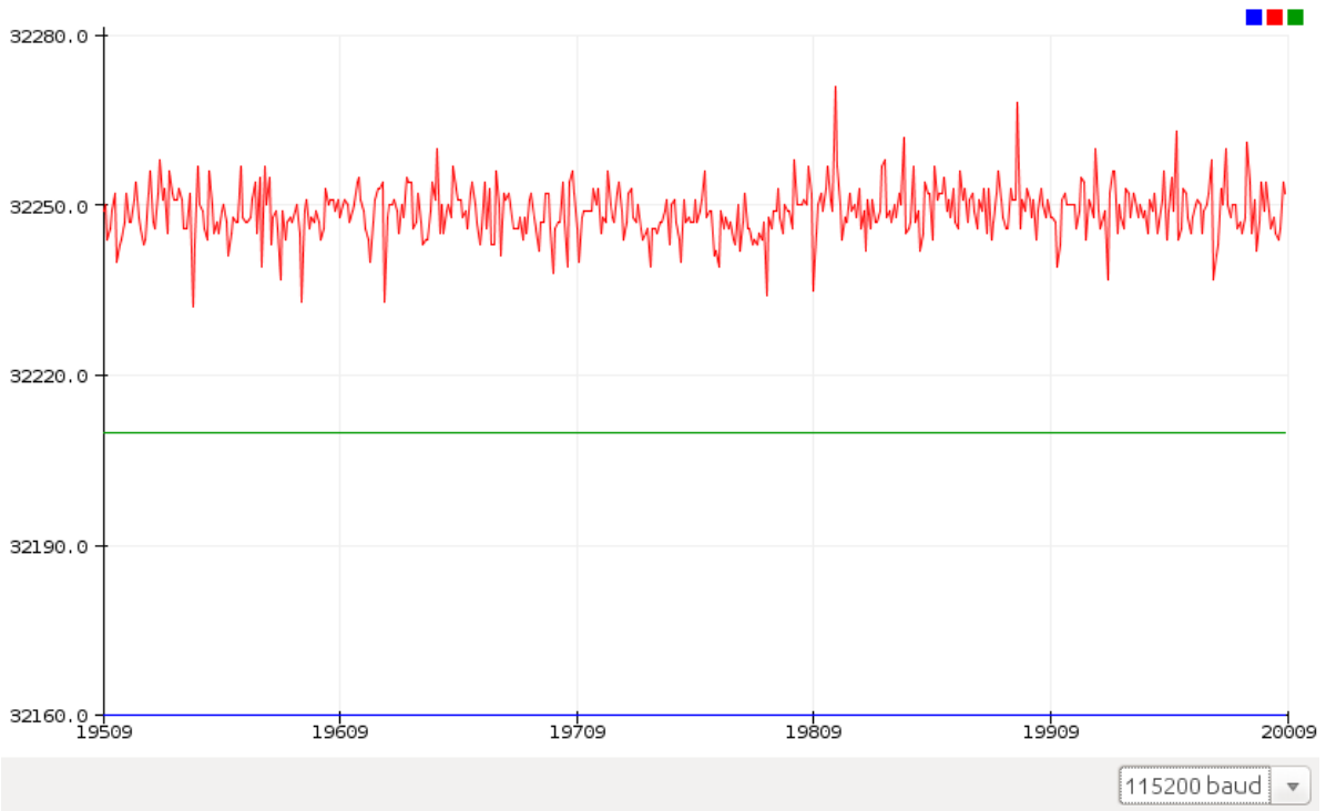
Figure I3: 16-sample averaging; high sampling speed; high conversion speed
