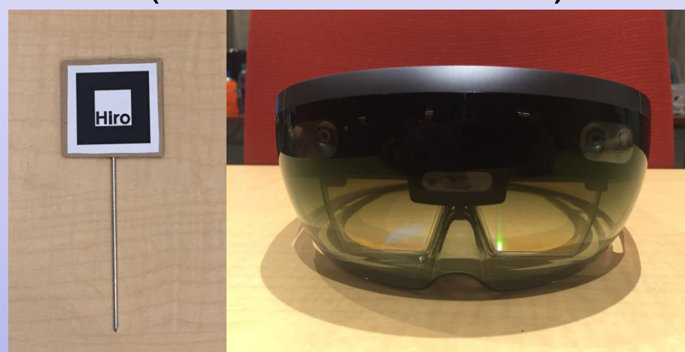
Figure 1: Surgical tool (left) and Locatable camera on HoloLens (right)
