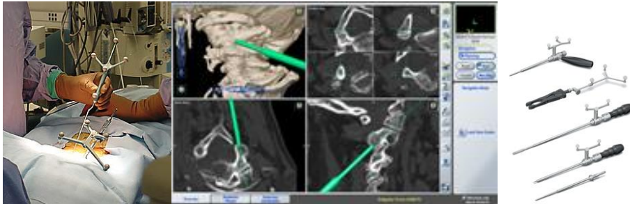
Fig. 3: Surgical Navigation for Spine Surgery. (Left) OR scene; (Middle) typical display; (Right) typical instruments. (Pictures are captured from web and show Brainlab system, but there are many similar systems).
