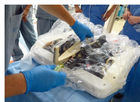
Drape robot, attach needle guide
